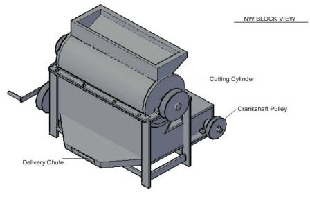
Fig. 1: Isometric drawing of orange juice extractor
